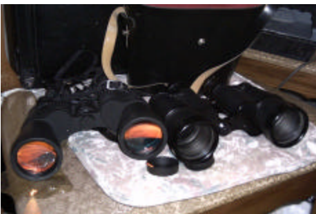
The author's Vivitar 7X50 and Charles Frank 10X50 binoculars. Note how the UV coatings on the Vivitars are quite bright and reflective – basically eliminating their use for astronomy except for viewing the moon.
